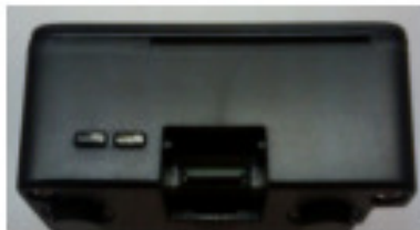
Front View: Status Lights & μSD slot
