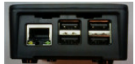
Rear view: Ethernet and USB Ports
